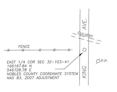
TIES: 56.54 NW TO PUNCH HOLE IN WEST END CULVERT 29.85' NE TO PUNCH HOLE IN WEST ENC CULVERT 45.25' SE TO PK IN POWER POLE
